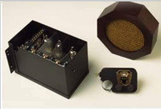
This reproduction of Motorola's first car radio, 1930's model 5T71, included (left to right) a radio receiver, tuning control and speaker.
